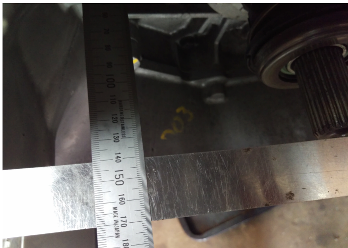
BELL HOUSING LENGTH 140mm
